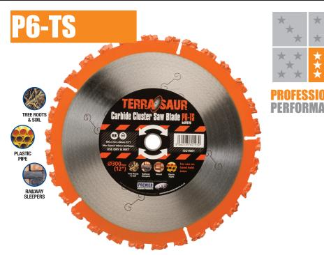
**DESCRIPTION:** The TERRASAUR is a tungsten carbide cluster saw blade that tackles jobs too tuff for a chainsaw or diamond blade. Hidden nails, screws and stones - no problem. The TERRASAUR is reversible, so if cutting speed reduces, turn the blade around and continue cutting. Unlike a diamond blade, the TERRASAUR blade cuts well then tilted and can withstand heavier pressure.
