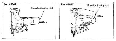
Refer to the table at right to select the proper speed for the workpiece to be cut. However, the appropriate speed may differ with the type or thickness of the workpiece. In general, higher speeds will allow you to cut workpieces faster but the service life of the blade will be reduced.
