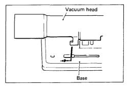
To attach the vacuum head on the tool, insert the hook of the vacuum head into the hole in the base. The vacuum head can be installed on either left or right side of the base. Then connect a Makita vacuum cleaner to the vacuum head.
