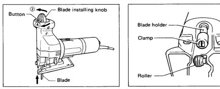
5. With the blade installing knob kept in this position, push it back down to its original position.
